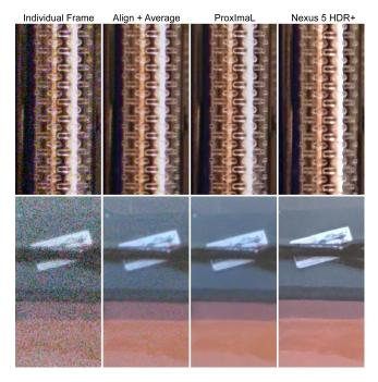
**Figure 8:** Burst denoising and demosaicking for images captured with a Nexus 5 cellphone camera. Averaging and aligning several frames mitigates noise, but does not achieve optimal results. We combine automatic image alignment, demosaicking, and burst denoising into a single inverse problem that shows similar or better performance than the Nexus 5's HDR+ application.
