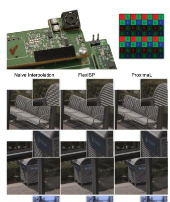
**Figure 7:** High dynamic range from a single RAW image. The sensor captures interlaced exposures via a coded rolling shutter (top right), often found in moderns sensors (e.g., Aptina AR1331CP and Sony IMX135). FlexISP demonstrated state-of-the-art reconstructions for these types of problems, but ProxImaL further improves recovered image sharpness, runtime, and convenience.<sup>2</sup>
