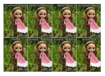
**Figure 9:** Comparison of image priors for burst denoising & demosaicking. For this simulation, a non-local means (NLM) prior outperforms the BM3D prior. The approximate NLM implemented in OpenCV is faster than, but not quite as good as, a full implementation.<sup>3</sup>
