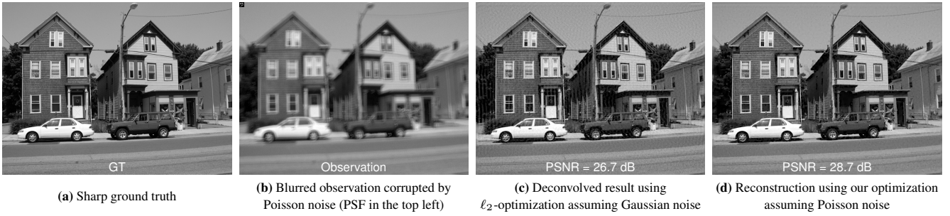
Figure 1: Effect of Poisson noise on deconvolution with large kernels: This example demonstrates that proper noise modeling leads to significant gains in reconstruction quality for large blur kernels. To only demonstrate the effect of the noise model, we did not use cross-channel information for this example. Since the Poisson distribution can be approximated well by a normal distribution for large values of the mean, the most significant improvements of using the proper noise model can be found in the low-intensity regions.
